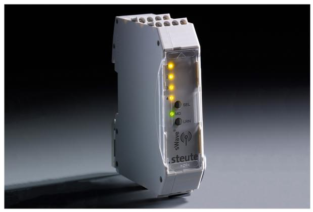
steute is launching a new wireless receiver RF Rx SW868-NET-4S-A 48V for its nexy wireless network, developed with a view to applications involving automated guided vehicles (AGV).
