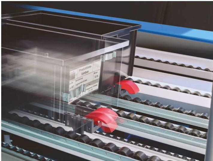
Fig. 4: This device (tilting sensor) was developed especially for eKanban applications
