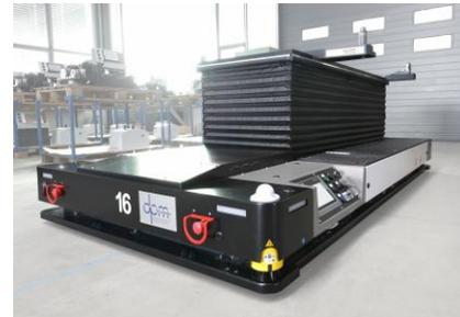
*The latest AGV generation for the automotive industry from dpm. Workers can ride pillion and assemble components at the same time.*
