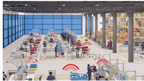
A wireless network can assume several tasks at once – for example, communication with an AGV fleet and replenishment of workstations via eKanban.
